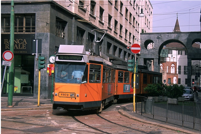
The most ecumenical location streetcars reach in the Duomo area nowadays is Piazza Fontana, just behind this view of a Route 12 4900-series "Jumbo" car on Via Larga. These units were built from 1976-8 in two series, by Fiat (the first 50) and Stanga. In this view of car 4875's left side, note that the cab is offset to the right side.
