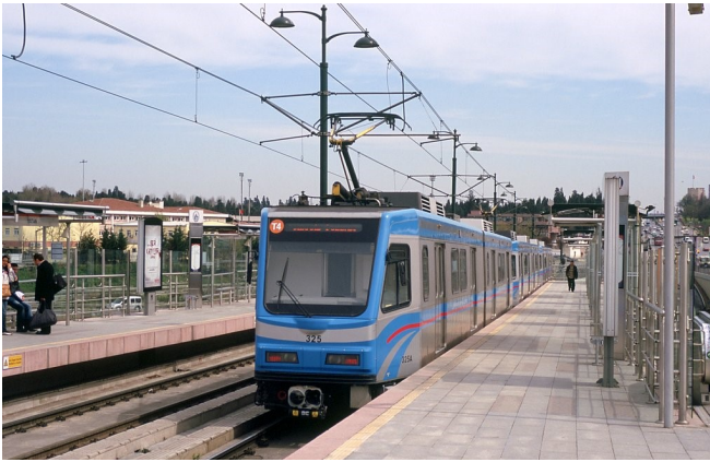
A second view of the elevated Vatan station, with an outbound train of Hyundai-Rotem cars. 34 of these cars were built in 2007 for the opening of the line, and provide the bulk of the service. Vatan is a transfer point to the M1 line, with the latter running in a subway at this point.
