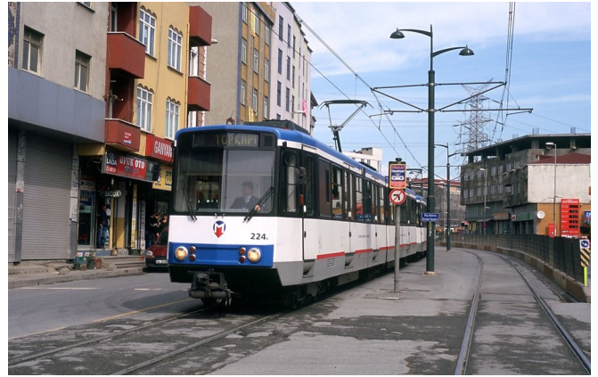
224 is one of the 1976 Duewag-built ex-Koln cars, which is set for high-level platform loading when used on the T4. It is shown on the tail track just beyond the temporary terminal of the light rail line at Mesoid-I Salam, on the outer section, where the line runs in a fenced-in center reservation in the middle of an arterial street.
