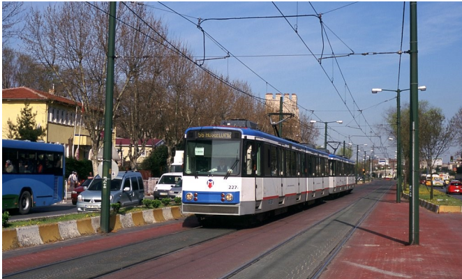
The other cars running on the T1 are Stadbahn B LRVs, built by Duewag for Koln in the 1970s and acquired by Istanbul in 2007. These cars are limited to tripper service over the heaviest part of the T1. 227 is shown running inbound in the center median of Turgut Ozal Cd approaching the Findikzade stop.
