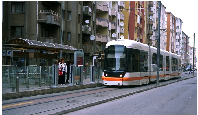
The single-track section of route 2 near the Marmure station. Note that only inbound cars will stop at this platform, as the rolling stock has doors only on the right side.
