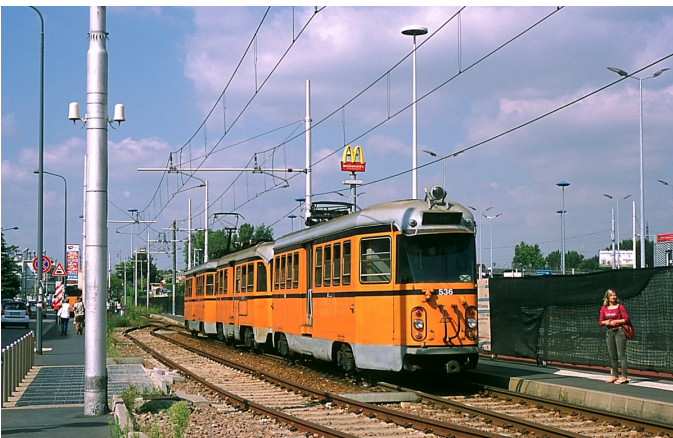
Two views of the 7-mile-long Milan-Limbiate interurban line. The only such line in service during 2014, its 3-car sets continue to trundle on. Oddly enough they are made up of two control trailers with pantographs sandwiching a blind motor. The cars were built for another interurban line (now replaced by metro line 2) in 1950-4, and were assembled together in 1964, a half-century before this visit. I cannot help loving them. The left view shows Maria waiting for a friend to join her aboard one of the interurban cars at its Comasino terminal. The right photo is of my outbound train waiting for the inbound to pass at the Cassina Amata Scambio stop, a little under halfway along the line.
