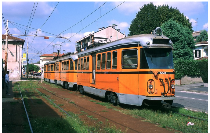
Two views of the 7-mile-long Milan-Limbiate interurban line. The only such line in service during 2014, its 3-car sets continue to trundle on. Oddly enough they are made up of two control trailers with pantographs sandwiching a blind motor. The cars were built for another interurban line (now replaced by metro line 2) in 1950-4, and were assembled together in 1964, a half-century before this visit. I cannot help loving them. The left view shows Maria waiting for a friend to join her aboard one of the interurban cars at its Comasino terminal. The right photo is of my outbound train waiting for the inbound to pass at the Cassina Amata Scambio stop, a little under halfway along the line.
