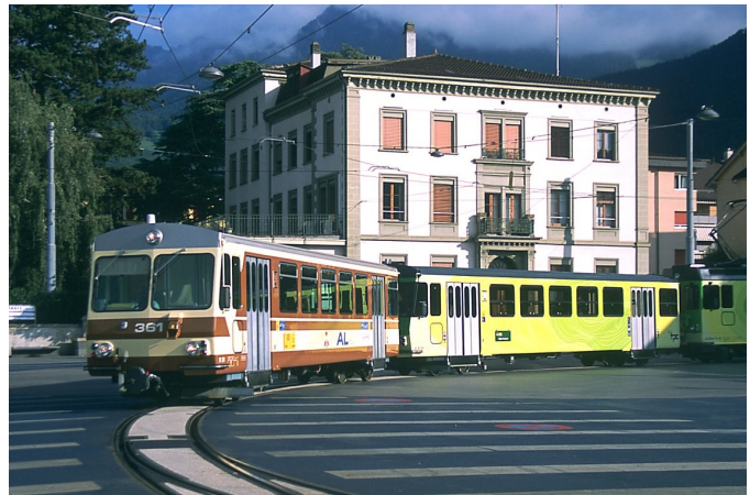
Left and right: These Control Trailer-Motor lashups are outfitted with the Abt rack equipment, the norm for the Aigle-Leysin line. Trailers 361 and 362 were built in 1987, and 363 (not shown) is identical but was constructed in 1993. Matching motors 311-313, respectively, were built in the same years by a consortium of Vevey (ASMV), Swiss Industrial Group (SIG) and Brown Boveri (BBC), prior to the rationalization of the car building industry that saw Stadler and Bombardier acquire the railcar assets of those companies. The left photo shows the TPC's new paint scheme on a train waiting at the station, while the scene at right shows a motor pushing two trailers as it enters the same station on a lazy Sunday morning.
