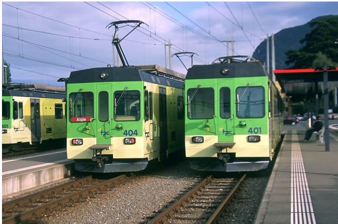
Left and right: Two views of the 400-series cars that run over the former Aigle-Sepey-Diablerets Line. There are four 1987-built motors on the roster, and they are usually paired with control trailers built in 1966 (but not necessarily on this Sunday morning). No longer do they load from the pavement of the forecourt of the CFF (SBB) railway station, but rather from regular railroad station platforms, as shown by the left photo. The view on the right shows operation along Avenue de Loes surrounded by a healthy display of poinsettias. The sky towards the west is threatening, but that weather never reached the eastern end of the Rhone Valley.
