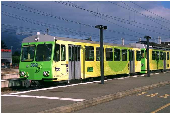
Left and right: These Control Trailer-Motor lashups are outfitted with the Abt rack equipment, the norm for the Aigle-Leysin line. Trailers 361 and 362 were built in 1987, and 363 (not shown) is identical but was constructed in 1993. Matching motors 311-313, respectively, were built in the same years by a consortium of Vevey (ASMV), Swiss Industrial Group (SIG) and Brown Boveri (BBC), prior to the rationalization of the car building industry that saw Stadler and Bombardier acquire the railcar assets of those companies. The left photo shows the TPC's new paint scheme on a train waiting at the station, while the scene at right shows a motor pushing two trailers as it enters the same station on a lazy Sunday morning.
