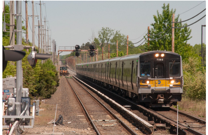
M-7 7383 (Bombardier Transportation, February, 2005) leads Train #2053 into the Central Islip station at 1:56 pm on February 21, 2018. In the distance, the remains of CI 2 Interlocking can be seen with home signals 1E and 2E now bagged, out of service. The switch at the east end of the former passing siding has already been removed.
