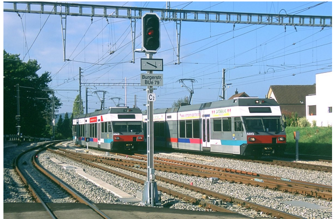
Two views of the BTI's modern 1997-built cars at Tauffellen. The left view shows a Biel-bound unit accelerating after pausing to drop and receive passengers. The right view shows the yard with two of the cars laying over before the afternoon rush hour. The BTI was the first recipient of these Stadler designed and built cars, which with their control equipment between two articulated sections, had become very popular in Switzerland. The diesel version was first placed in service on NJ Transit's River Line.
