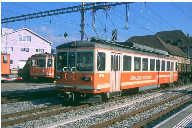
Units from the 300-series are used as backup for the BTI's regular passenger service and for powering freight trains. The series was built between 1966 and 1978 by Schlieren-Oerlikon for the Solothurn-Niederbipp Bahn, which was merged with the BTI to form the Regionalverkehr Oberaargau, which later expanded into the current Aare Seeland Mobil (ASm). I was lucky to see the freight pass by while waiting to continue my journey to Ins.
