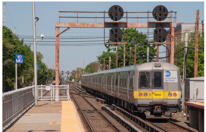
M-3 9930 (Budd-General Electric, July, 1986) leads Train #2056 east out of the Farmingdale station at 4:06 PM on May 21, 2018, right about on time. Enjoy the traditional position light signals while you can. All of the interlockings from here to Ronkonkoma are getting six-aspect Reduced Aspect Signaling dwarf signals (made by Safetran actually). Farm 1 Interlocking here will be renamed simply Farm as Farm 2 is being renamed PW. PW is what Farm 2 (at the end of the original double track, east of the old Republic station) was called before the electrification in 1987-8.
