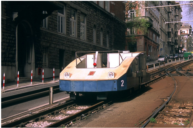
Views at the foot of the funicular showing new (2005) tractor 2 and the stub switch in both its positions. The trough guiding the cable is also shown.
