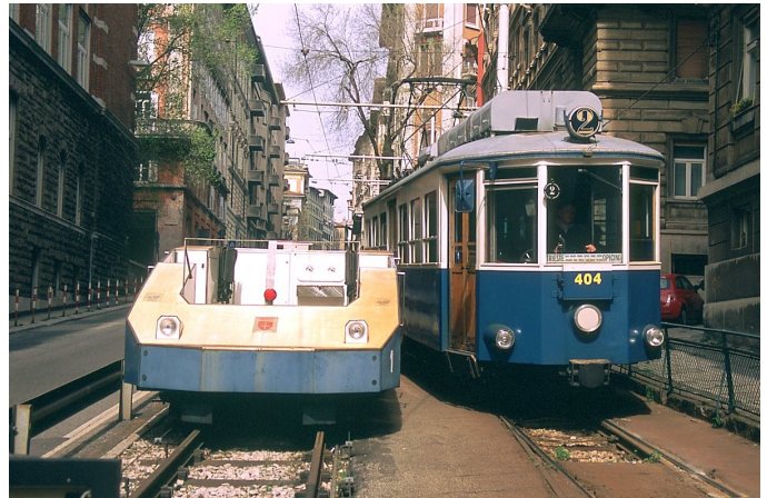
Streetcar 404 has taken the switch at the foot of the funicular and is now heading for downtown Trieste. Tractor 1 is alongside on the "siding," having just completed its service as a buffer for the passenger car as it descended. It will wait for 404 to return so it can push the tram back up.
