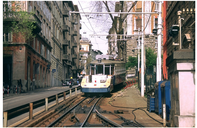
Views at the foot of the funicular showing new (2005) tractor 2 and the stub switch in both its positions. The trough guiding the cable is also shown.
