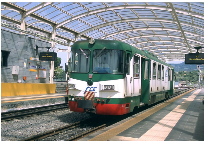
Our outbound class ADE 11-20 railcar pauses at the Adrano Nord station, waiting for a similar unit heading for Catania to pass. These DMUs were built by Stanga in 1980 and constitute the Circumetnea's largest group of rolling stock. Note that the track area in this attractive modern station is sufficiently wide to allow for the line's eventual conversion to standard gauge.
