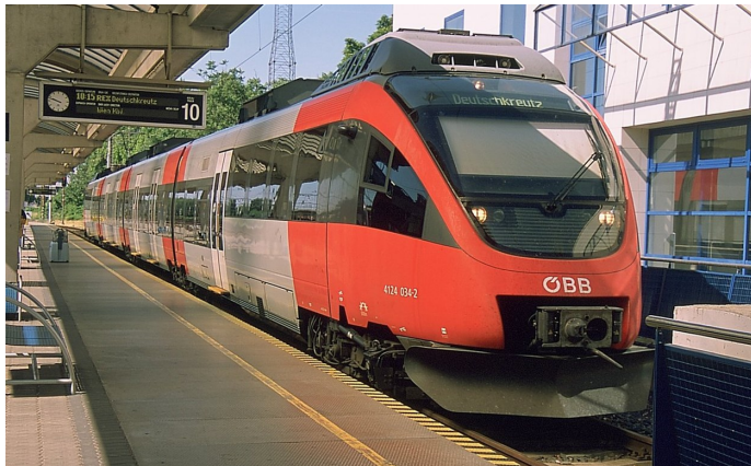
The dual-voltage eMU that brought me from Vienna to Bratislava at a bumper block in Petrzalka station. The Bombardier Talent eMU is already signed up for its return trip to Deutschkreutz via Vienna.
