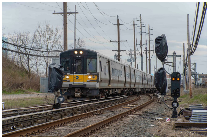
M7 7651 (Bombardier Transportation, 5/2006) is seen here leading Train #861 from Long Beach to Penn Station through Lead Interlocking, east of the Island Park station. This portion of the interlocking controls the end of double track. The new color light signals are still bagged out of service in this view south on April 14, three days before the signal cut-in.
