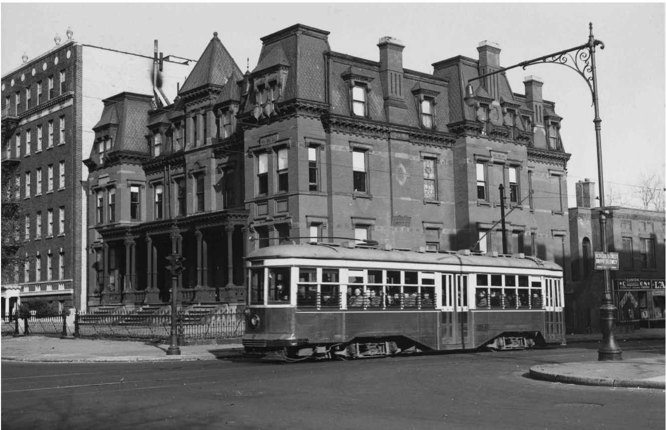
Peter Witt 8473 (Osgood-Bradley, 1925) is westbound on DeKalb Avenue at Washington Avenue. It's November 18, 1947 and this DeKalb Avenue car will in due time arrive at its Sands Street terminal.
