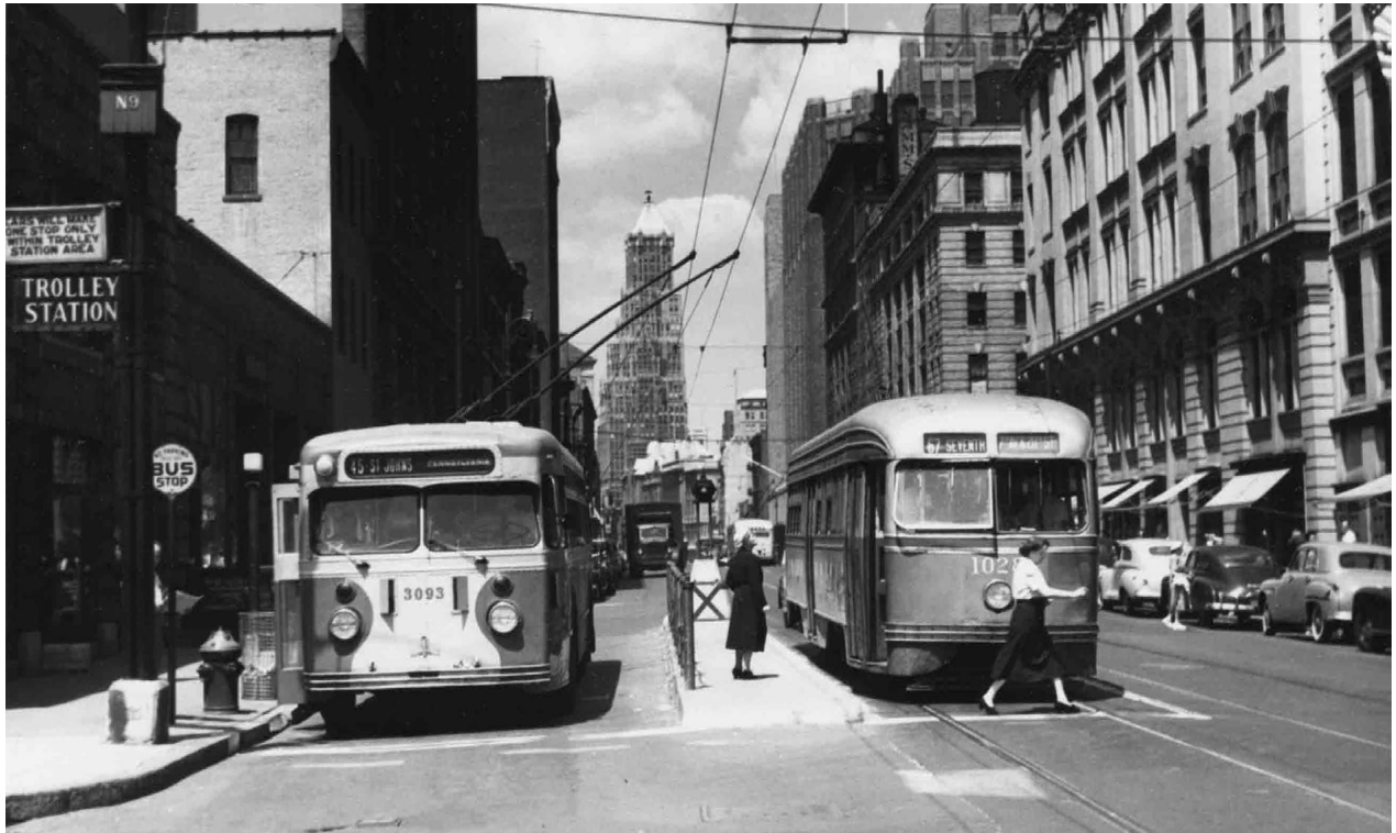
A multi-modal scene on Livingston Street & Bond Street in Downtown Brooklyn. PCC 1028 (St Louis Car, 1936) is on the 67-Seventh route and is destined for 7th Avenue & 20th Street at the south end of Park Slope. Trolley coach 3093 (St Louis Car, 1948) is on the 45-St. Johns route and will terminate at Pennsylvania Avenue in East New York. The date is July 21, 1950.
