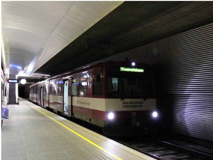
GT8NF 58 (SGP, 2002) at the terminal under the Hauptbahnhof in Salzburg on October 31, 2020. This car had been rebuilt from a GT6 in 2013. 21-72 photo via Urban Electric Transit
