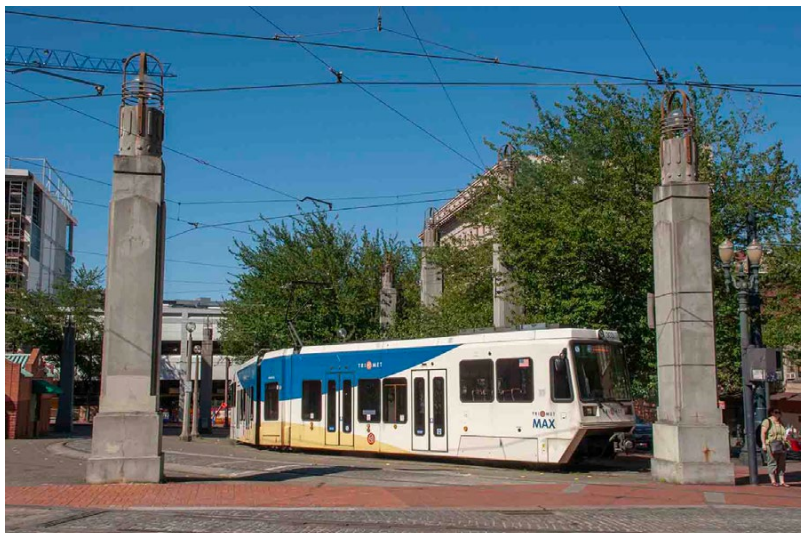
(Below) The third batch of LRVs are represented here by Type 3/SD660s Nos. 303+322 (Siemens, 2003). This set was not in revenue service at this point. It is pictured on the short-turn loops west of the Galleria/SW 10th stop, at SW 11th Avenue & SW Yamhill Street.
